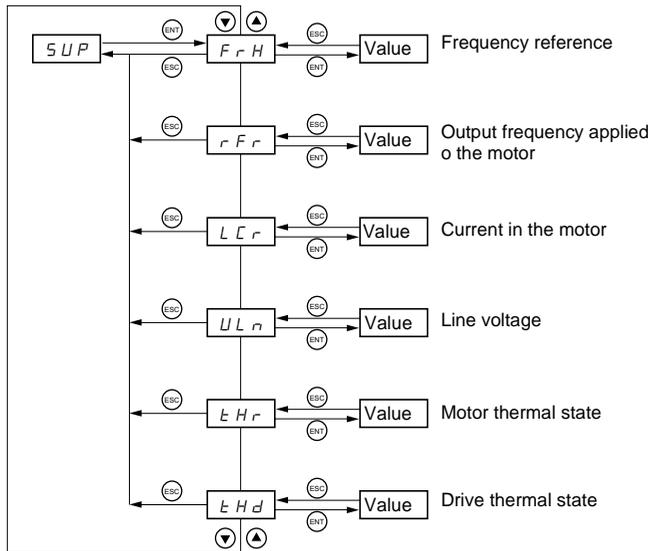
When the drive controller is running, it displays the value of one of the monitoring parameters. The default display is frequency reference (parameter FrH).
