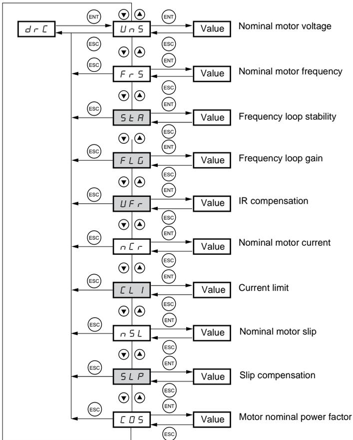
**Table 14: drC Motor Control Parameters**
