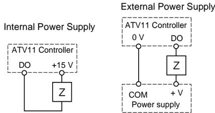
If a logic output is assigned, Z is an external device such as a low-voltage relay. If an analog output is assigned, Z is an external device such as a meter.
